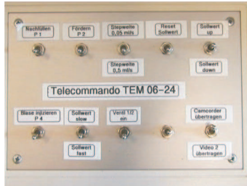
Fig. 17.13. User panel for TEM0624. During the flight the experiment was operated manually via telecommand with this panel
